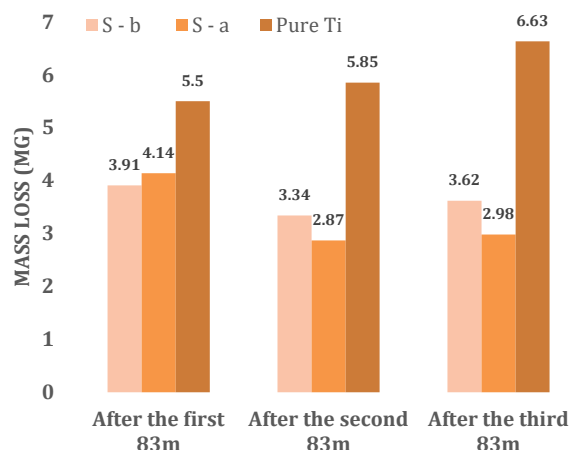
Figure 3. Weight loss due to wear
